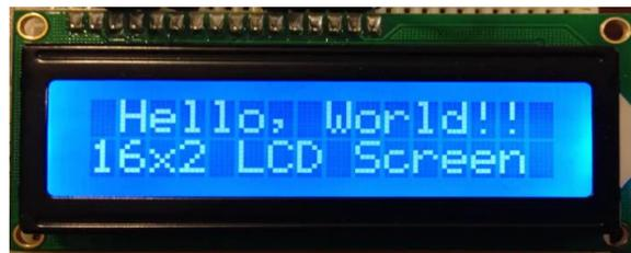
**Gambar 2** LCD 16 x 2
