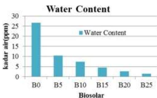
**Gambar 4.** Pengaruh Biosolar Terhadap Kadar Air (Water Content)
