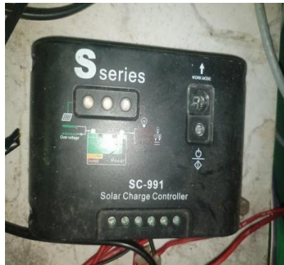
Gambar 4. Solar Charge Controller
